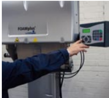
Step 1: The operator chooses a pre-programmed bag setting.
