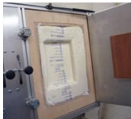
Step 4: After a few seconds the FOAMplus® cushion is ready.
