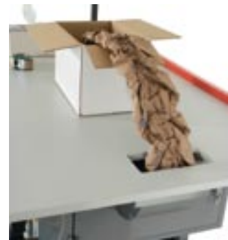
Standard single packing table with PAPERplus® Classic under the table. Extras include AIRplus® Mini on a shelf, a carton rack, and a computer rack with TFT monitor connector.
