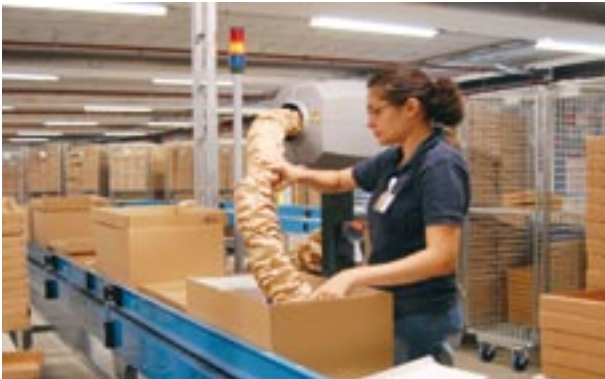
In-line packaging using a Chevron machine.
